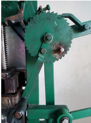
Figure 10. Actual Diagram of Ratchet and Pawl
