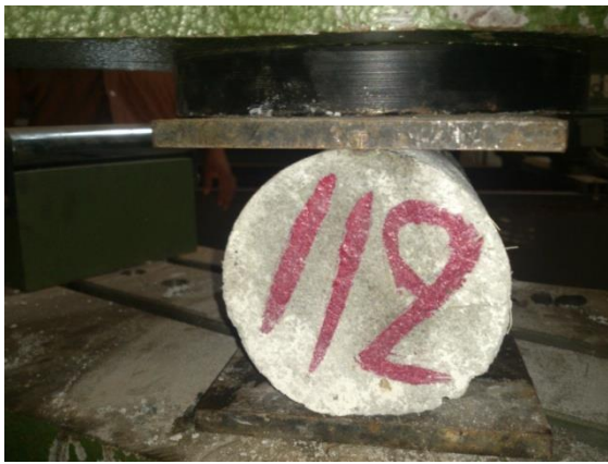
Figure 5.3. Split tensile test
