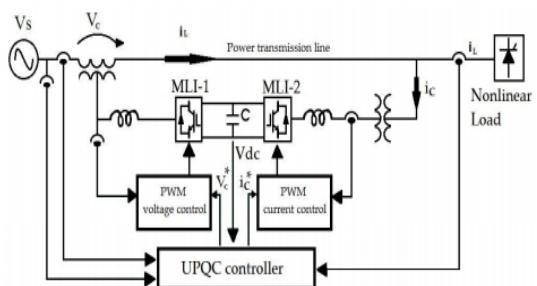
**Figure 1.** conventional UPQC under steady state
