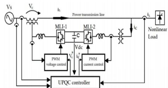
**Figure 1.** conventional UPQC under steady state
