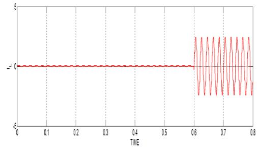
**Figure 10.** Load Neutral Current
