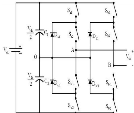
**Figure 2.** Diode clamped type configuration for multilevel VSC
