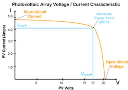
Figure 1. V-I characteristics of solar array in light radiation intensity variation
