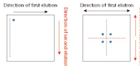
**Figure 4:** 2-D development on a planar OPLC column. Dotted lines correspond to solvent inlet microchannel. Blue corresponds to sample, and white, black, and red are the sequential development
