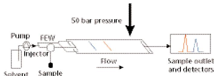
**Figure 5:** Concept of FEW with the distribution of solvent at sample channel and flowing walls.
