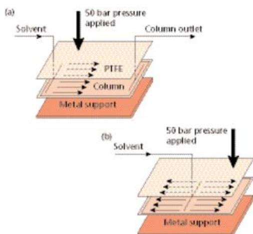
**Figure 3:** OPLC cassette design for (a) linear one-dimensional and (b) bidirectional chromatography separations steps.
