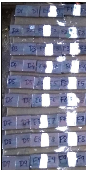
Figure 5. Application of flux between two plates to be welded
