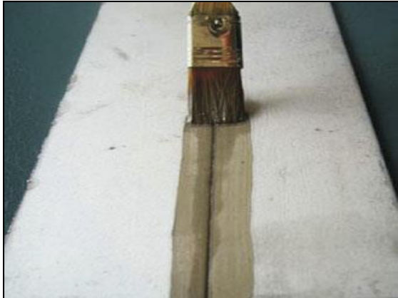
Figure 4. The application of flux
