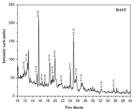
**Figure 2.** Powder XRD pattern of DAST nanorods
