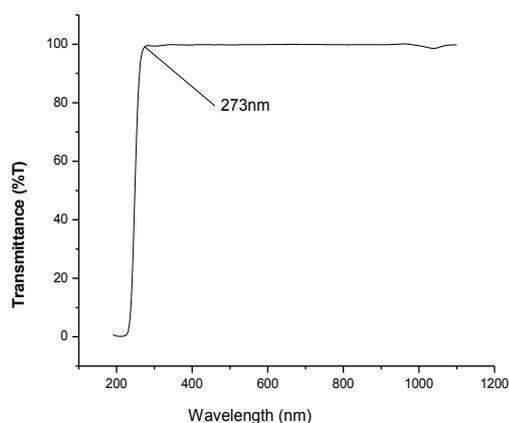
**Figure 3.** UV-Visible spectra of TFAG crystal
