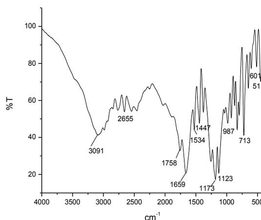
**Figure 2.** FTIR spectra of TFAG single crystal
