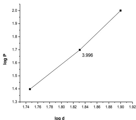
**Figure 7.** Work hardening coefficient curve of TFAG crystal
