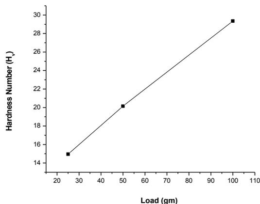
**Figure 6.** Hardness variation of TFAG crystal
