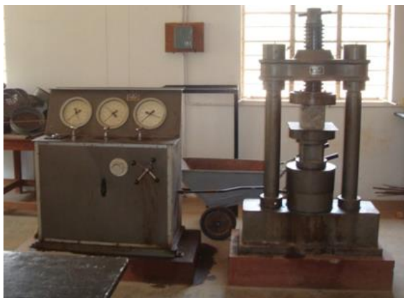
Figure 1. Compression testing machine.
