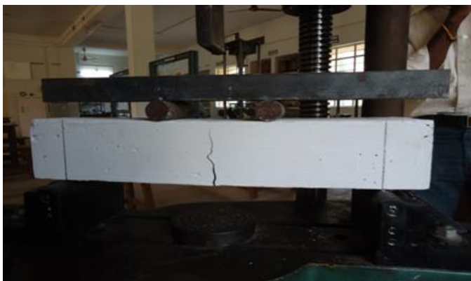
Figure 4 Illustration of fracture of failure specimen.
