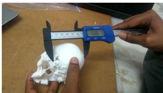
Figure 10. Distance measured between Inion-Porion of the fractured side of the skull before operation using digital vernier callipers
