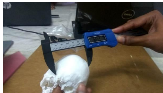
Figure 11. Distance measured between Inion-Porion of the fractured side of the skull after operation using digital vernier calipers
