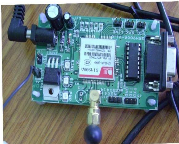
Figure 6. GSM SIM900 Circuit
