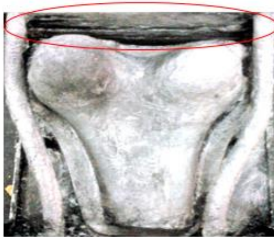
Figure 8. Poor Deposition on the Vertical Surfaces
