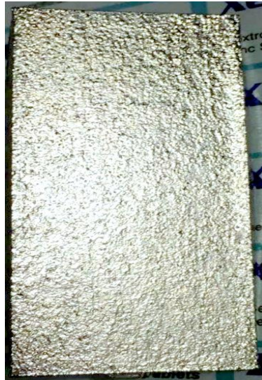
Figure 4. Sample with Poor Adhesion
