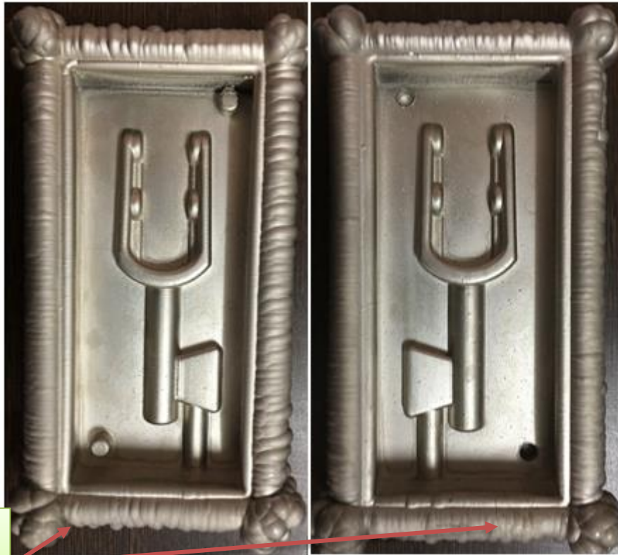
Figure 5. Electroformed with lumps of additional mass
