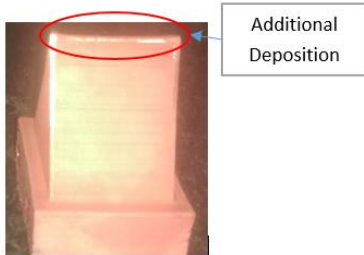
Figure 6 (b). Excessive Deposition due to the Sharp Edge as High Current Density Area
