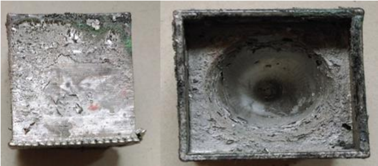
Figure 3. Burnt Samples Due to High Current Density during Nickel Deposition
