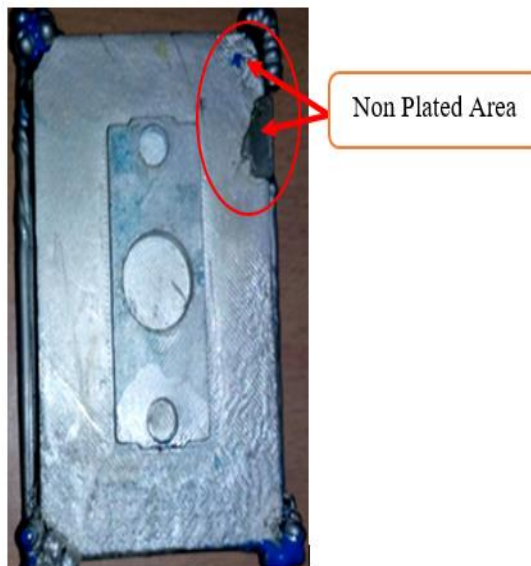
Figure 2. Uncover Area due to Poor Conductivity
