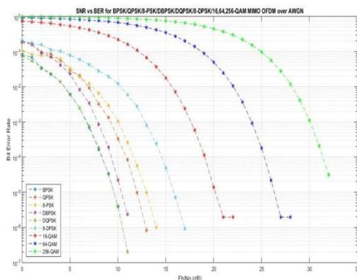
**Figure 6.** SNR vs BER for different modulation over AWGN
