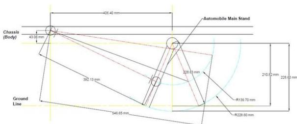
**Figure 5.** line diagram of the main stand
