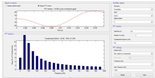
Figure 11. THD analysis of output voltage of single phase five level cascaded H-bridge multilevel inverter with filter. (THD=21.53%)
