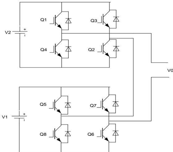
**Figure 2.** Five level cascaded H-bridge multilevel inverter
