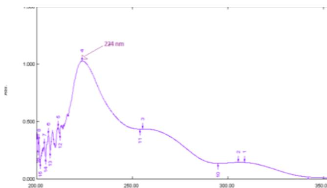
Figure 1: Absorption maxima of candesartan cilexetil in phosphatebuffer pH= 6.8
