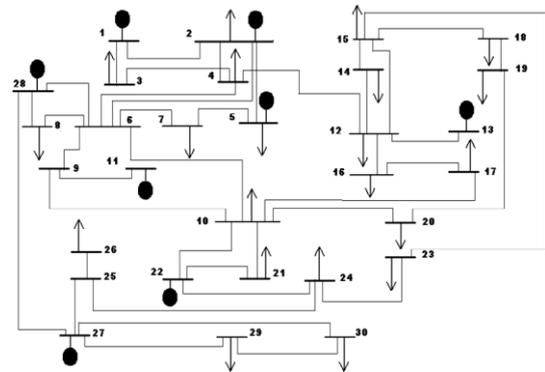
Figure 2. Single Line Diagram of IEEE 30 bus test system
