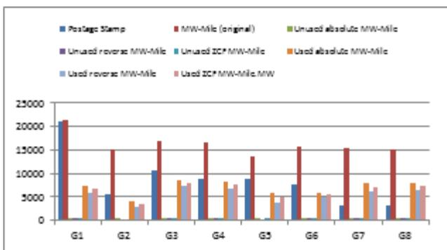
**Figure 4.** Transmission Pricing based on different pricing methods at Generator Buses when load demand is actual
