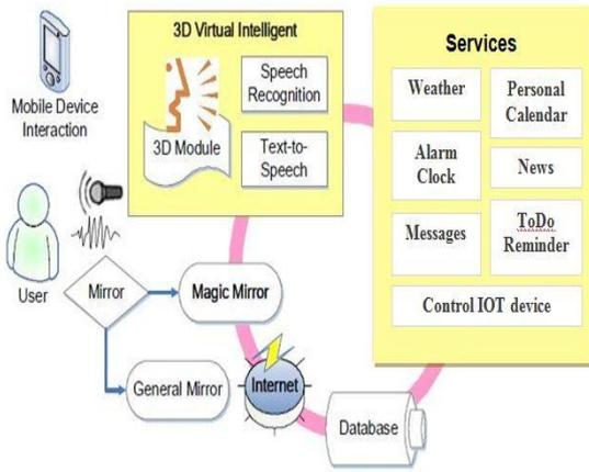
**Figure 2.** Function diagram of Hermione 1.0-mirror
