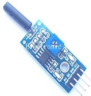
Figure 6. Vibration Sensor
