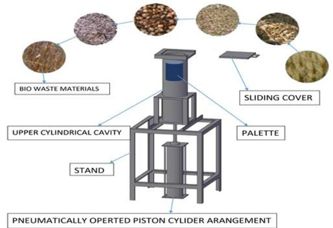
Figure 4. Simple Model of Pallet Making Machine
