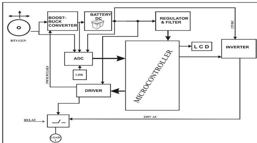
Figure 2. Working diagram of electrical power generation by using RTV.
