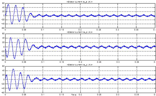
**Figure 5.** Simulated Stator Current Of A SPWM VSI Fed To A Induction Motor.
