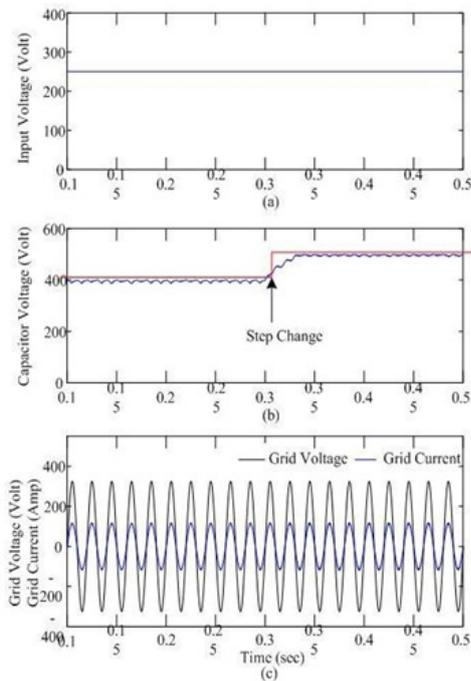
**Figure 4.** Simulation result for step change in capacitor voltage from 400V to 500V (a) Input voltage (b) Capacitor voltage (c) Grid voltage and current (scaled by x 10).
