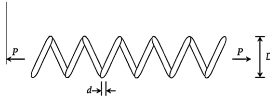
Figure 6. Schematic of tension/compression spring design problem
