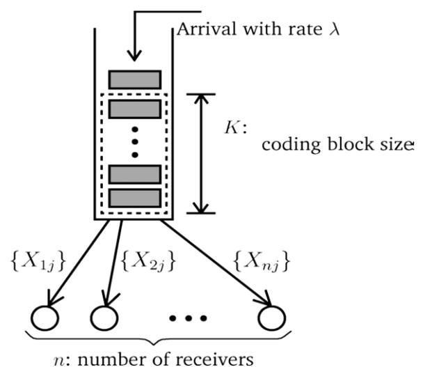
**Figure 1.** Broadcast with Discrete-Time Queuing Model.
