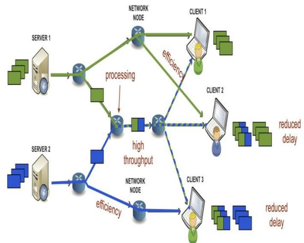
Figure 2. System architecture for throughput rateless code.
