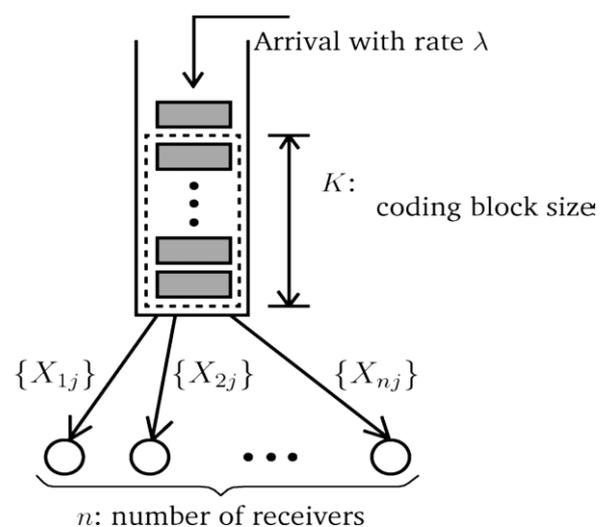
**Figure 1.** Broadcast with Discrete-Time Queuing Model.
