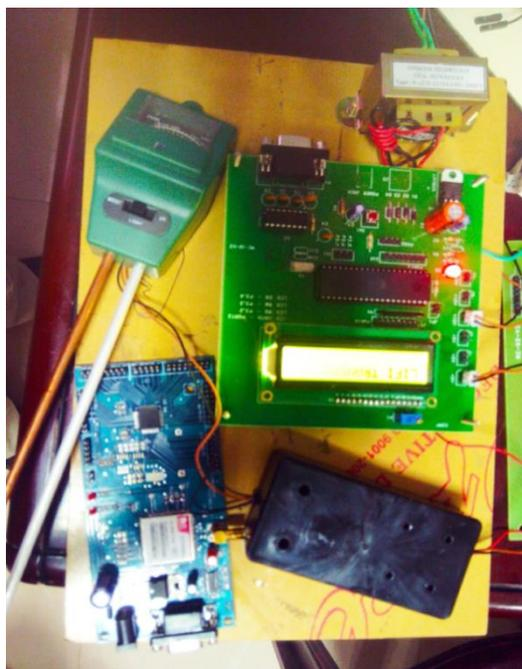
**Figure 3.** Board of the Water Management System
