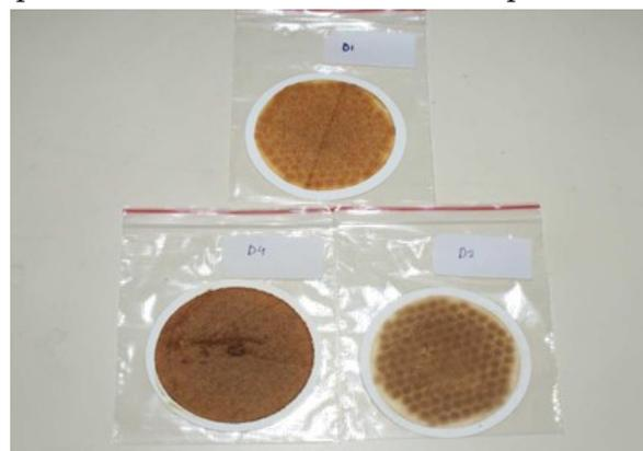
**Figure 3.** Brown carbon loaded quartz filter paper
