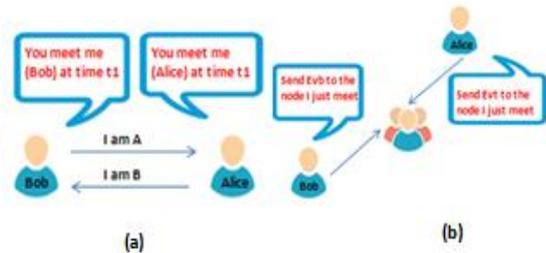
**Fig. 1. General solution for encountering record collection. (a) Create the encountering evidence under neighbor node anonymity. (b) Route the encountering evidence to the other node after separation.**
