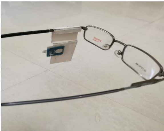
Figure 4. Sensor module on the frame of the spectacle
