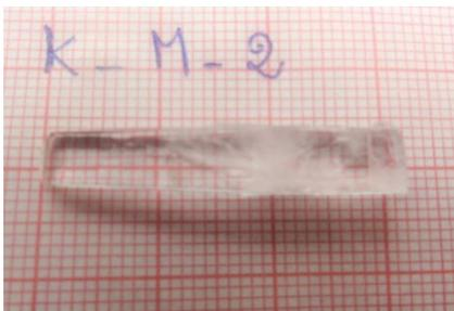
**Figure 1.** As grown single crystal of LMKDP
