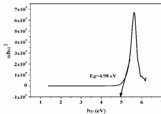
Figure 7. UV-vis band gap of LMADP Crystal.
