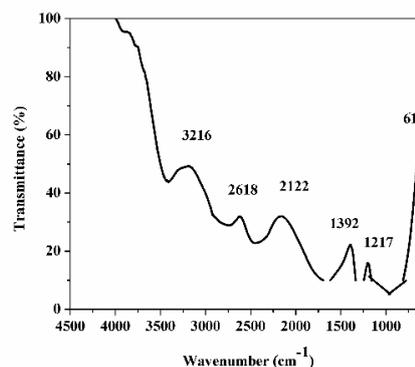
**Figure 3.** FT-IR spectral analysis of LMKDP Crystal.
