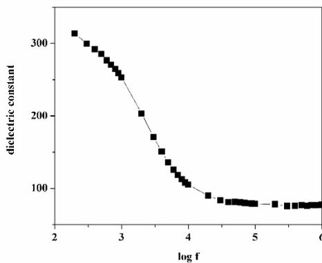
**Figure 4.** Dielectric constant Vs Log f of LMADP Crystal
