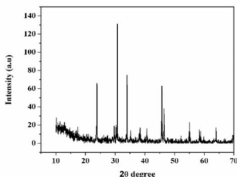
**Figure 2.** Powder XRD pattern of LMKDP crystals.
