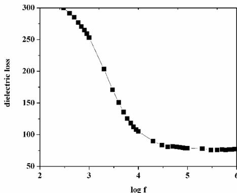
Figure 5. Dielectric loss Vs Log f of LMADP Crystal.
