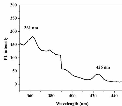
**Figure 9.** Photoluminescence Emission spectra of LMKDP crystal
