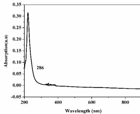
**Figure 6.** UV-vis absorption of LMADP Crystal.
