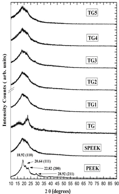
**Figure 3.** XRD pattern of virgin PEEK, SPEEK, TG and SPEEK/TG composite membranes
