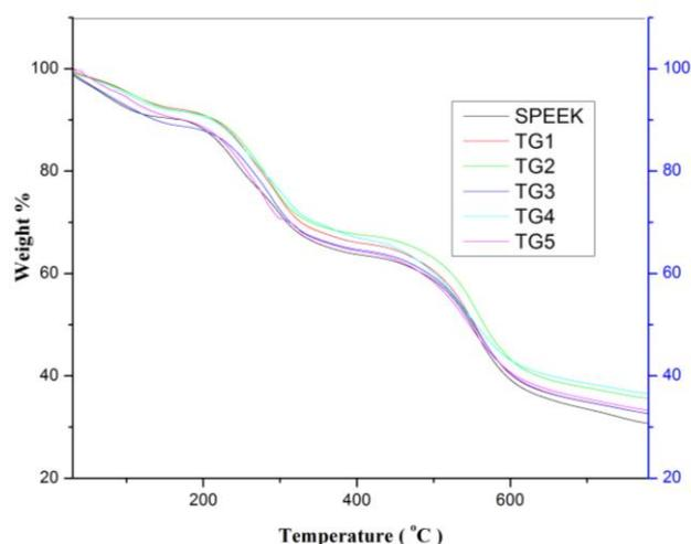
**Figure 6.** TGA of pristine SPEEK and SPEEK/TG composite membranes.
