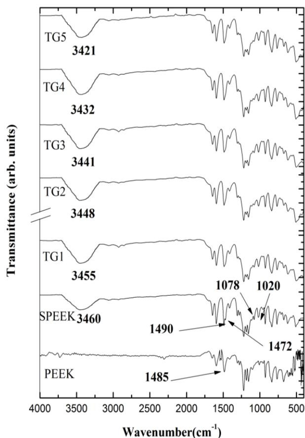
**Figure 5.** FTIR spectra of PEEK, SPEEK and SPEEK/TG composite membranes.
