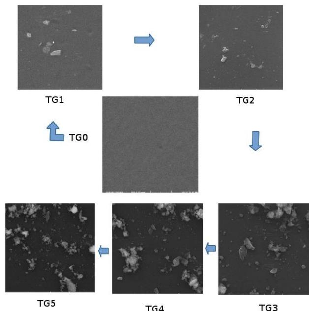
**Figure 4.** SEM images of pristine SPEEK, and SPEEK/TG composites.
