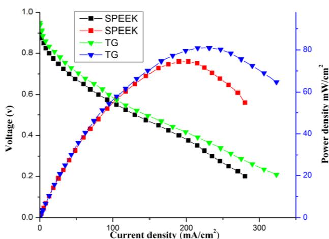
**Figure 8.** Single cell performance studies for virgin SPEEK and SPEEK/TG composite membranes
