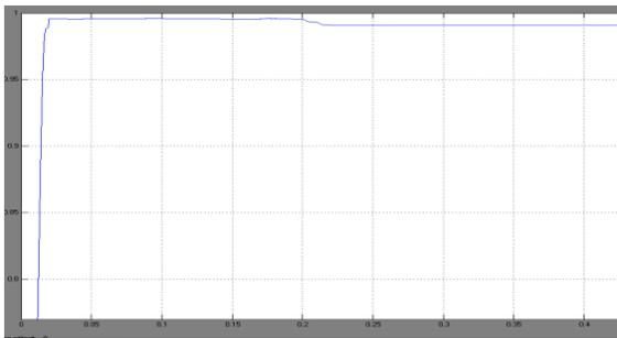
**Figure 12.** PCC Voltage with DSTATCOM during LG fault
