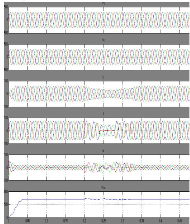
Figure 7. Simulation results for Linear RL Load
