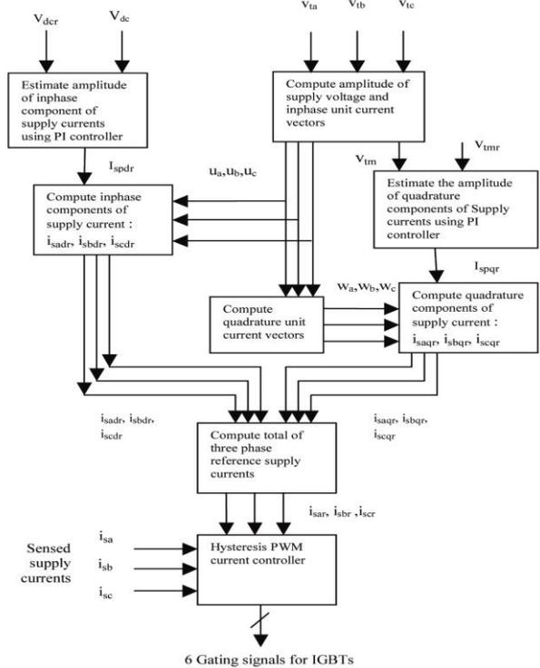
**Figure 2.** Control method for DSTATCOM
