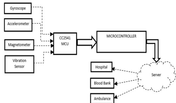
Figure 9. Block diagram for detecting accident.
