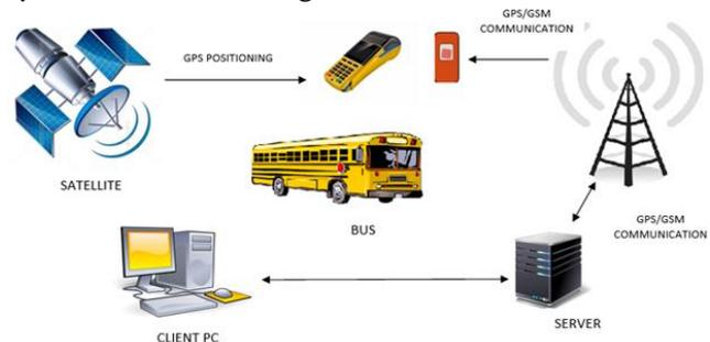
Figure 5. Bus tracking system Architecture
