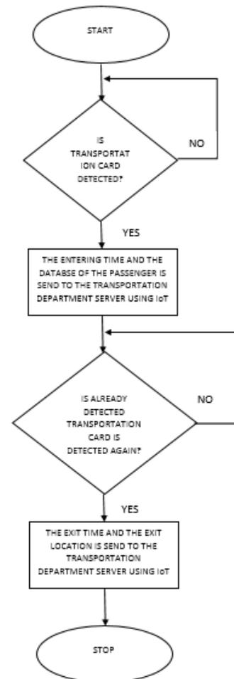
**Figure 6.** flow chart for sending the passenger details to the server
