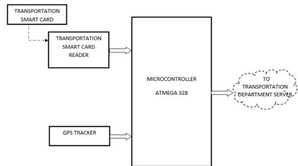
Figure 8. Block diagram of Passenger identification and theft identification system
