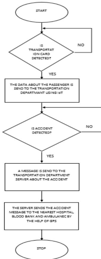
Figure 7. Flow diagram for the accident detecting and reporting methodology
