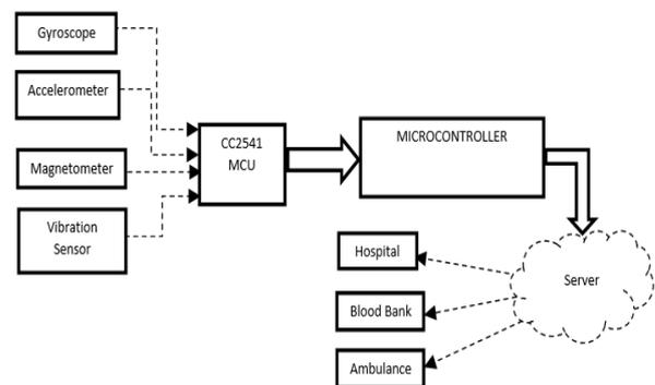
Figure 9. Block diagram for detecting accident.
