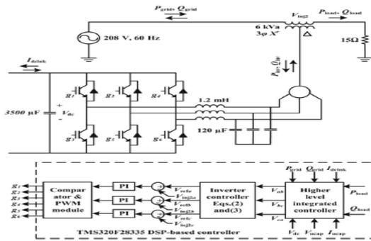
**Figure 2.** Model of three-phase series inverter (DVR) and its controller with integrated higher order controller.
