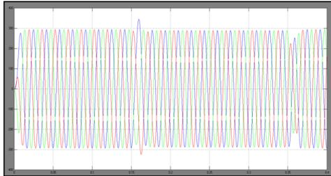
Load voltages  $V_{Lab}$  (blue),  $V_{Lbc}$  (red), and  $V_{Lca}$  (green) during sag
