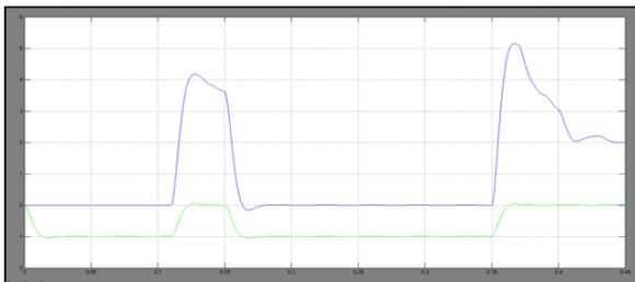
Currents of dc-dc converter during voltage swell
