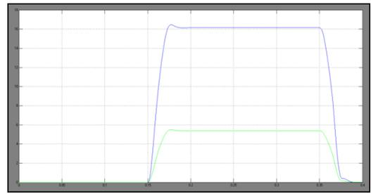
Voltages of dc-dc converter during voltage sag
