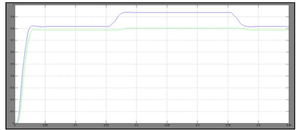
Active power of grid, Load and inverter during voltage swell
