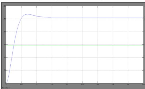
Voltages of dc-dc converter during voltage swell
