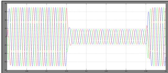
Source voltages  $V_{sab}$  (blue),  $V_{sbc}$  (red), and  $V_{sca}$  (green) during sag
