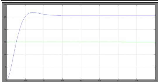
Source and load RMS voltages  $V_{srms}$  and  $V_{Lrms}$  during sag
