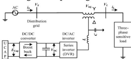
**Figure 1.** One-line diagram of DVR with UCAP energy storage.
