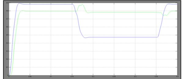
Currents of dc-dc converter during voltage sag
