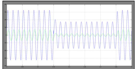
$V_{inj2a}$  (green) and  $V_{sab}$  (blue) waveforms during sag
