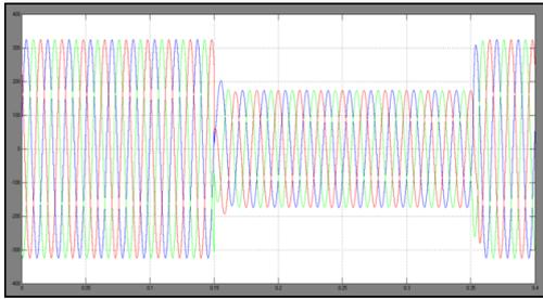
Injected voltages  $V_{inj2a}$  (blue),  $V_{inj2b}$  (red), and  $V_{inj2c}$  (green) during sag
