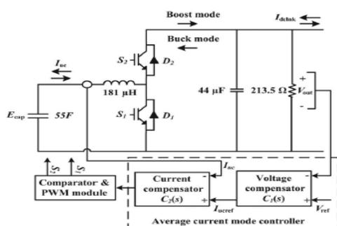
Figure 3. Model of the bidirectional dc-dc converter and its controller.
