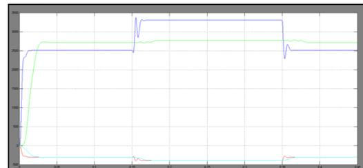
Active power of grid, Load and inverter during voltage swell
