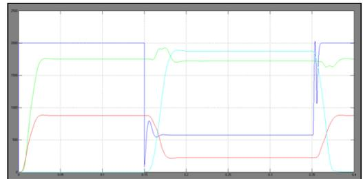
Voltages of dc-dc converter during voltage sag
