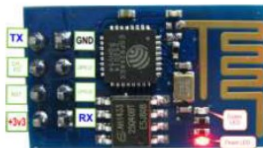
Fig 2: ESP8266 Pin Details
