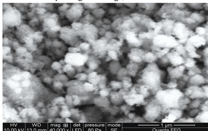
**Figure 3.** SEM image of the as prepared CeO<sub>2</sub> nanoparticles
