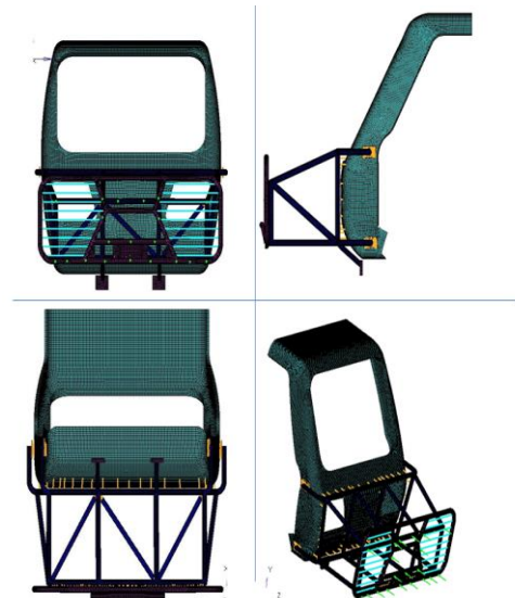
figure 2. describes the finite element bumper car assembly in different 2D views with different nodal structure.
