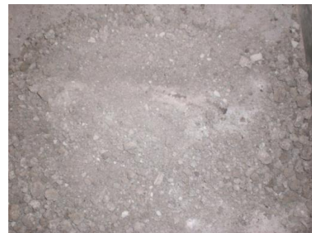
Figure 2. Mixing of soil-fly ash- industrial waste
