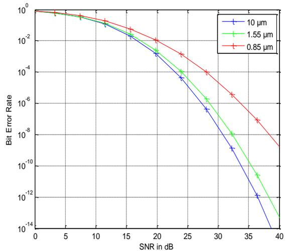
**Figure 5.** BER versus SNR for different wavelengths
