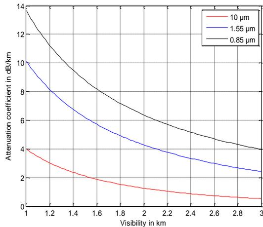
**Figure 3.** Wavelength Attenuation in dependency of wavelength
