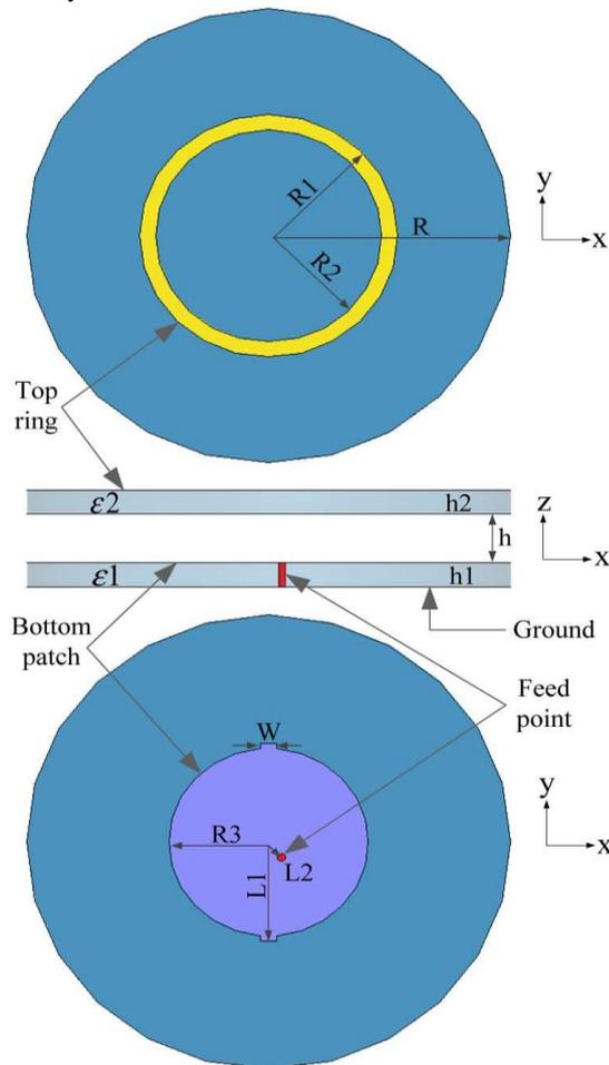
**Figure 1.** Geometry of the wide-beam circularly-polarized microstrip antenna
