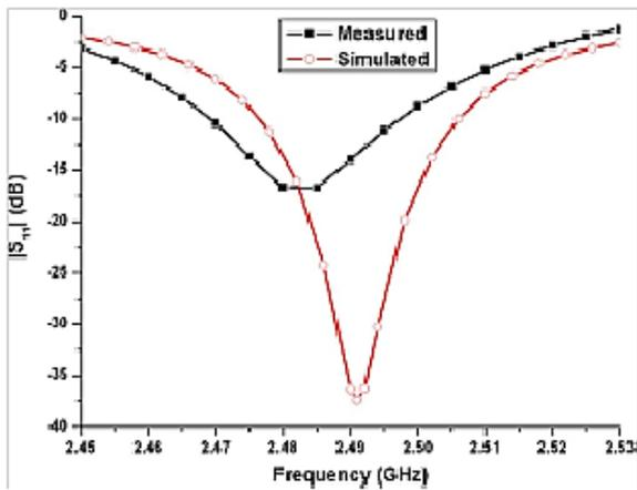
Figure 4. S11 for the proposed antenna
