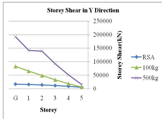
**Figure 5:** Storey shear profile in transverse direction
