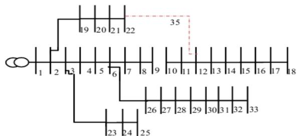
**Figure 3 :** single line diagram of 33bus test system after reconfiguration
