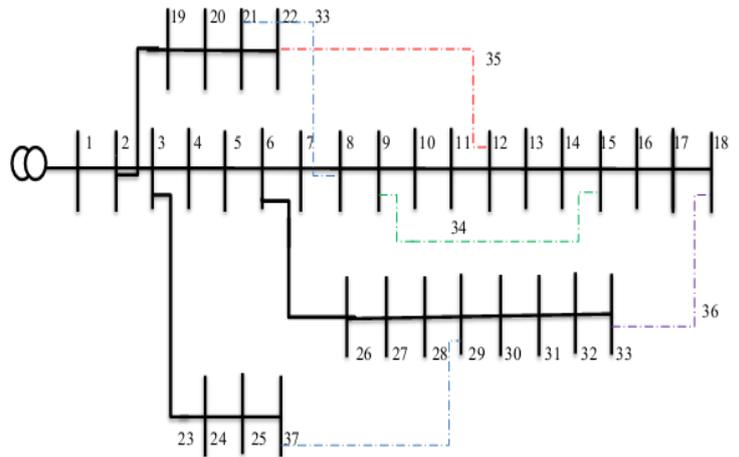
**Figure 2:** single line diagram of 33bus test system
