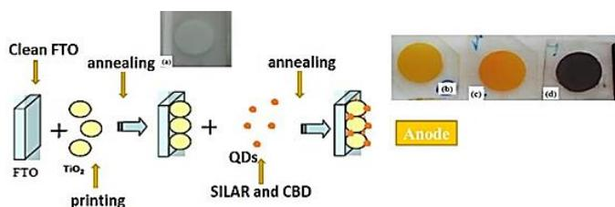
**Figure 1.** Schematic of photoanode structure.
