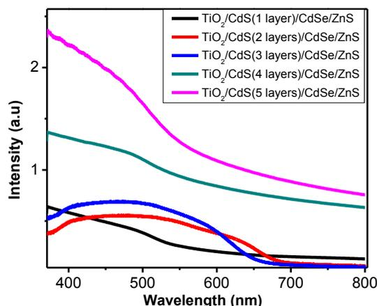
**Figure 3.** The UV-Vis of the TiO<sub>2</sub>/CdS/CdSe/ZnS photoanodes.
