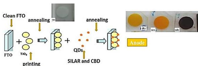
**Figure 1.** Schematic of photoanode structure.
