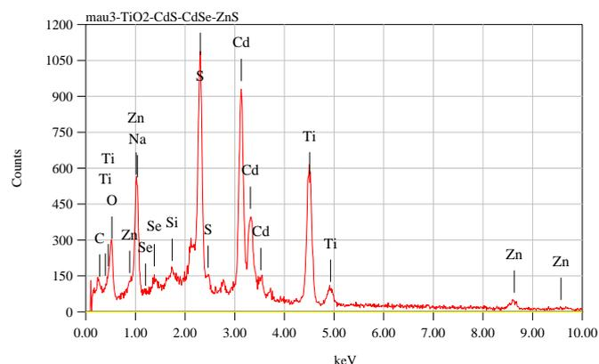
**Figure 2.** (a) The SEM image and (b) the EDS of the  $\text{TiO}_2/\text{CdS}/\text{CdSe}/\text{ZnS}$  photoanode.
