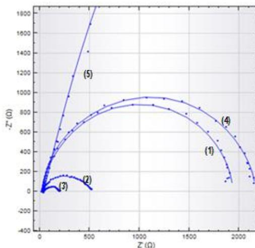
**Figure 4.** (a) The I-V curves and (b) the Nyquist plots of the QDSSCs with the different photoanodes.
