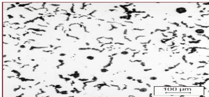
Fig.1.2: CGI GJV450 Microstructure
