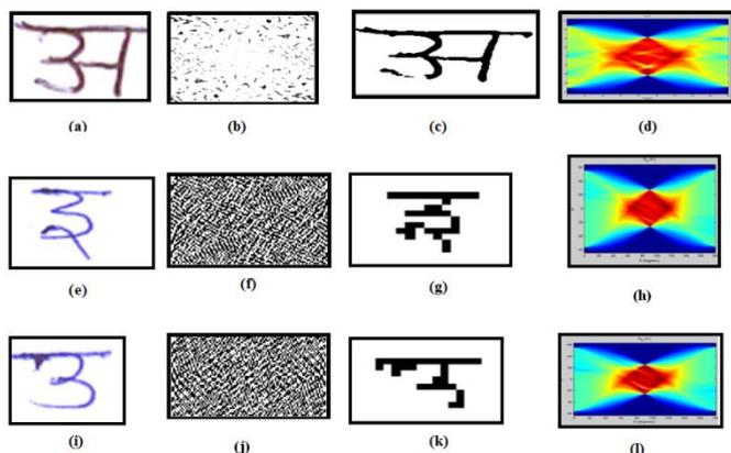
**Figure 3:** Results of feature extraction methods: (a) Image of character v, (b) DFT of character v, (c) DWT of character v and (d) Radon transform of character v, (e) Image of character b, (f) DFT of character b, (g) DWT of character b, (h) Radon transform of character b, (i) Image of character m, (j) DFT of character m, (k) DWT of character m and (l) Radon transform of character m.
