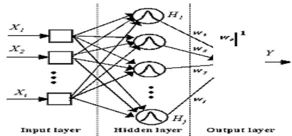
**Figure 4:** Radial Basis Function Network
