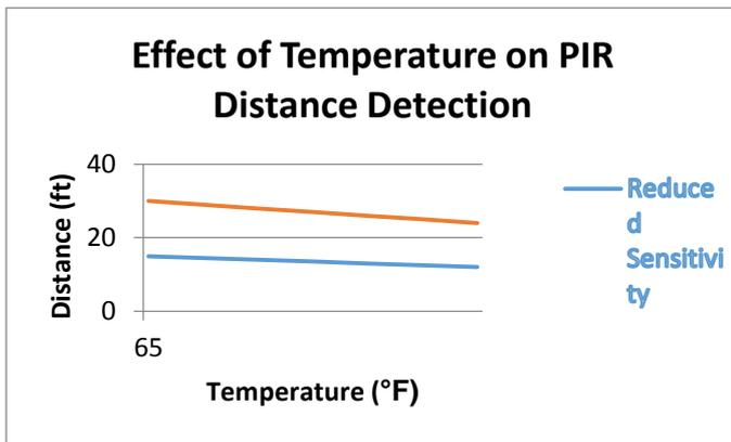
**Figure 3 :** Effects of temperature on PIR Sensor
