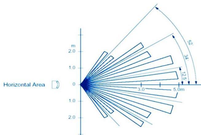
**Figure 2:** Pyroelectric sensor field of view
