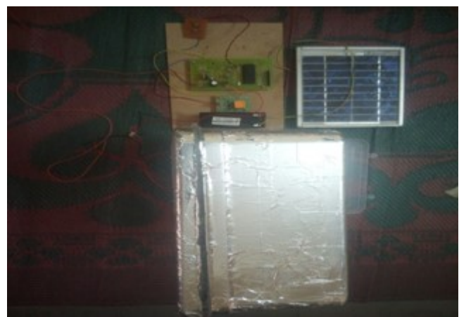
Figure 2. TEC assembled to cooling cabin
