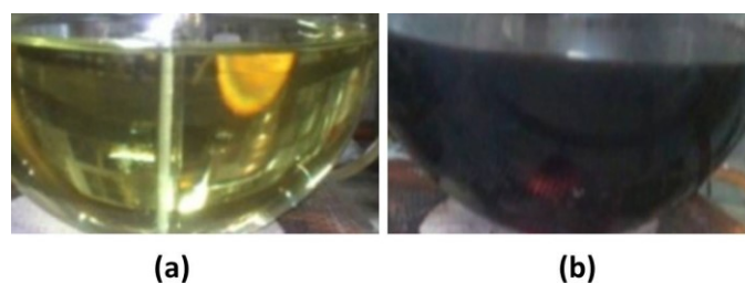
Figure 2. The change in sequence of the color of the reduction reaction during gold nanoparticle formation. (a) After some time during boiling the liquid changed to pale yellow color. (b) At the end of reaction the color was changed to blackish purple color.
