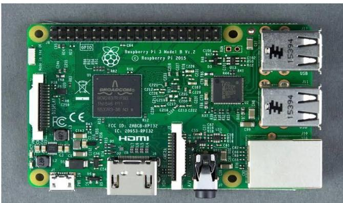
Figure 4. Raspberry pi 3 model b
