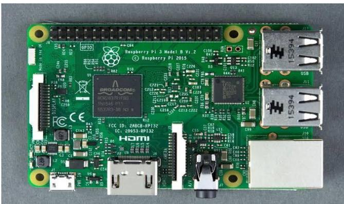
Figure 4. Raspberry pi 3 model b
